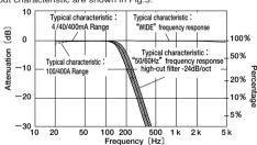
Fig.3 Model 2432/2433 Frequency Characteristic
