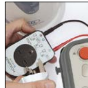
Class 1 PAT testing with the PAT Adapter1
