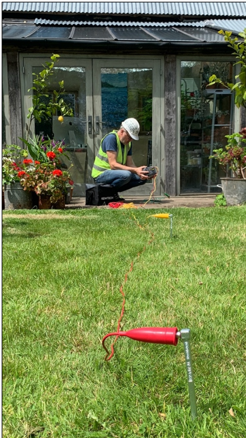
The Kewtech KT65DL Multifunction instrument with earth resistance testing kit.
